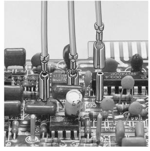
This terminal is used with 2.36mm diameter GT pins. The SPF terminal has a large contact area, withstands stress caused by repeated insertions and removals, and provides excellent retaining force. It is best suited for circuit connections that require a large current.
