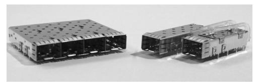
As data rates exceed 2.5 Gb/s, there is a greater need for higher EMI suppression. Enhanced EMI spring gaskets are added to the SFP cages to meet increased EMI requirements at higher data rates. The SFP Cages with enhanced EMI Gaskets are compatible with the existing SFP MSA panel cutout. The enhanced EMI gaskets provide increased contact area for improved EMI suppression.
