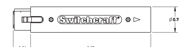
S3F5M 3 PIN FEMALE TO 5 PIN MALE DMX ADAPTER
