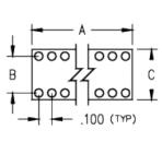
**Description:** DIP Header Interconnect Open Frame Through Hole Plating Code: **Shell Plating:** 10 μ" Gold over 100 μ" Nickel **Packaging:**
