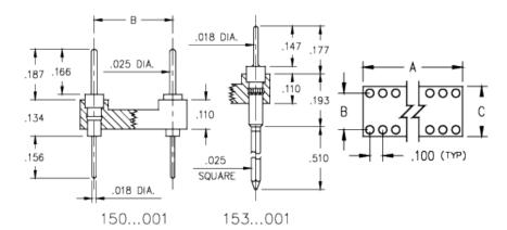
**Description:** DIP Header Standard Header 3 Level Wrapost Tail Open Frame Through Hole Plating Code: 10
