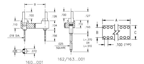
**Description:** DIP Header Slotted Header Solder Tail Open Frame Through Hole Plating Code: 10 Shell Plating:
