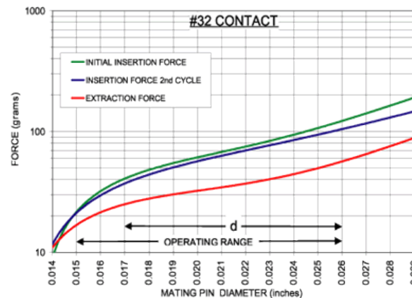
The insertion/extraction/normal force characteristics above were derived using a 30 microinch gold plated contact and polished steel gauge pins having a bullet-shaped tip.
