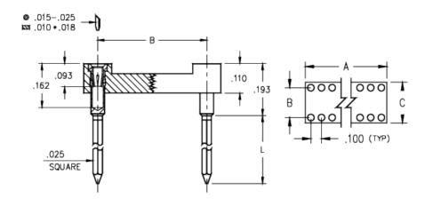
**Description:** DIP Socket Wrapost Tail 3 Level Wrapost Tail Open Frame Accepts .015-.025" Leads Plating Code: Shell Plating: 200 μ" Tin (matte finish) over 100 µ" Nickel
