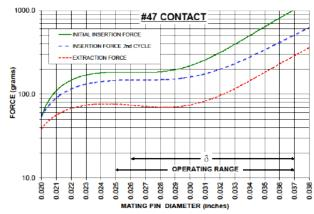
cteristics above were derived using 30 microinch gold plated contact and polished steel gauge pins having a bullet-shaped tip.
