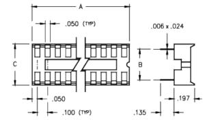
Description: DIP Socket Solder Tail Stamped and Formed Open Frame Through Hole Plating Code: 90 Shell Plating: 200 μ" Tin/Lead(93/7) over 100 μ" Nickel Packaging: Packaged in Tubes
