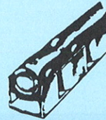
2. Insulation being pierced.
