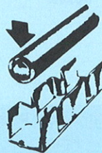
1. Prior to conductor insertion.
