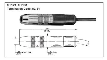
ST121: Straight Extension Jax® jack is a shielded 2-conductor jack with .50" (12.7 mm) outside diameter. Cable clamp connects shield or second conductor to cable. Mates with .25" (6.35 mm) diameter Switchcraft 2-conductor plugs.
