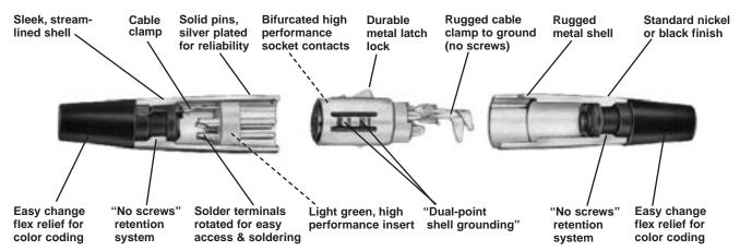
QGP connectors (3 contacts only) feature Vel-Tone® non-reflective finish, gray TPR flex relief and plated pins/contacts for the most demanding applications.
