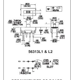
RECOMMENDED PC BOARD LAYOUT (Component Side)
