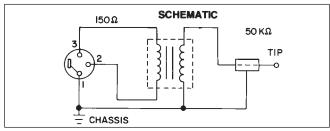
Series 9000 Line Matching Transformers offer low-loss interconnections between high and low impedance equipment. Exclusive mu-metal shielding protects against spurious electrostatic and RF fields. Units are bi-directional and can be used as follows:
