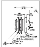
Rear of panel mount; 2 through 5 pins (male) or 2 through 5 contacts (female). Also 2-, 3- and 4-contact inserts with 2 shunted (N.C.) contacts. Mounting locknut (Part Number SL01), lock washer (Part Number SL02), and flat washer (Part Number SL03) supplied.
