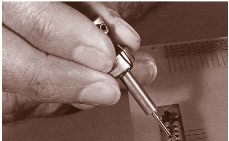
INSERT EXTRACTION TOOL WITH PLUNGER RETRACTED
