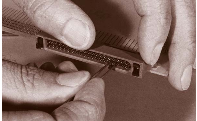
REMOVE DAMAGED CONTACT
