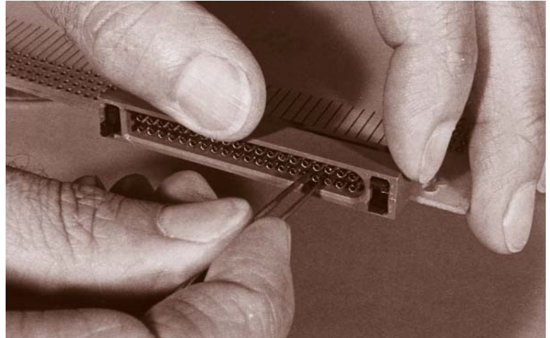
REMOVE DAMAGED CONTACT
