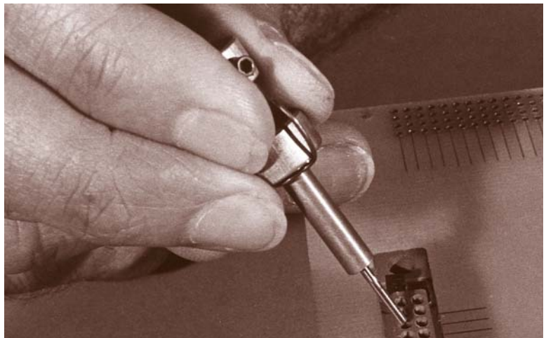
INSERT EXTRACTION TOOL WITH PLUNGER RETRACTED
