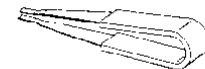
Contact Insertion Tool (For inserting contacts applied to small diameter wire) Part No. 91002-1 IS 408-7347
