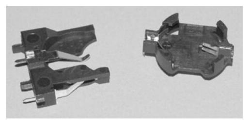
Tyco Electronics Top Load Battery is a high reliable receptacle for coin-cell (BR 2032 and CR2032) batteries. These batteries are used as battery back-ups in computers to store the RTC (real time clock) and other CMOS RAM data when the computer is not turned on. It can also be used in a variety of other electronic equipment needing a compact low wattage (typically less than 2Watts) battery source.
