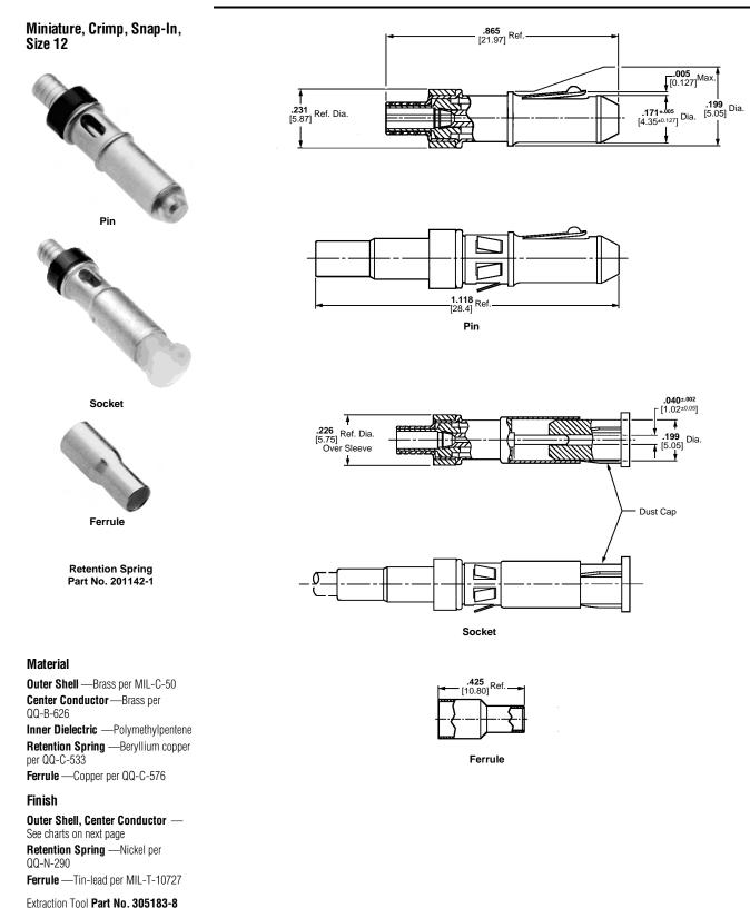
Dimensions are in inches and millimeters unless otherwise specified. Values in brackets are metric equivalents.
