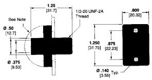
Note: Customer must protect back end against arc-over and breakdown if bulkhead and mounting hardware are metallic and at ground potential.
