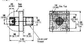
Note: If the panel or mounting hardware is at ground potential, guard against arcover and breakdown within the area defined by this line.
