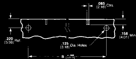
Recommended Pc Board Mounting Dimensions
