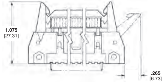
Figure 1 — Use Long Latch for AMP-LATCH Novo Receptacles with Strain Relief & Female Socket Connectors with Strain Relief
