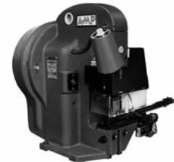
AMP-O-LECTRIC Bench Machine with Special Applicator
