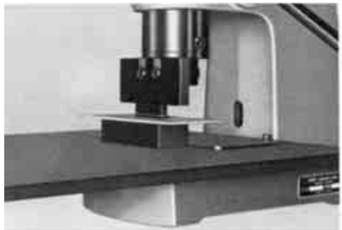
5. Press handle down gently and insert connector into the board.
