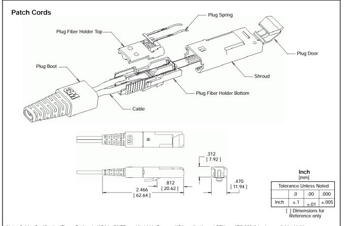
Note: Cable "Certification/Flame Rating" in USA is ONFR per UL 1666. For non-USA applications, LSZH per IEC 332-3 is also available. Volition VF-45 Patch Cords connected with Volition VF-45 Sockets perform to the following loss and reflection data and conform to the following combination of TIA, IEC and 3M performance specifications.
