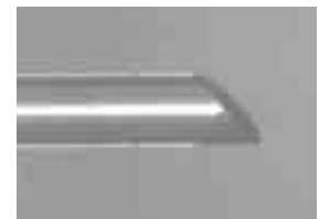
Straight and Angled Cleave
