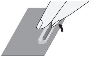
2. Securely insert the FPC so that it is perpendicular to the connector and horizontal to the connector.
