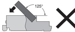
3. Lock and unlock the slider using the center of the slider. Using the end of the slider may result in incomplete locking, damage, or contact failure.
