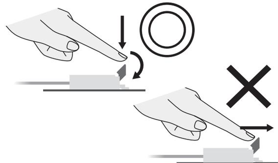
4. When unlocking the slider (lever), place your fingers on either side or the entire slider (lever) and slowly lift the slider (lever) up and away.
