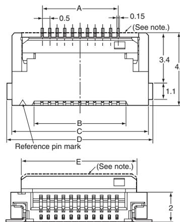
Note: Dotted lines indicate the shape and dimensions of 55-pin or 60-pin connectors.
