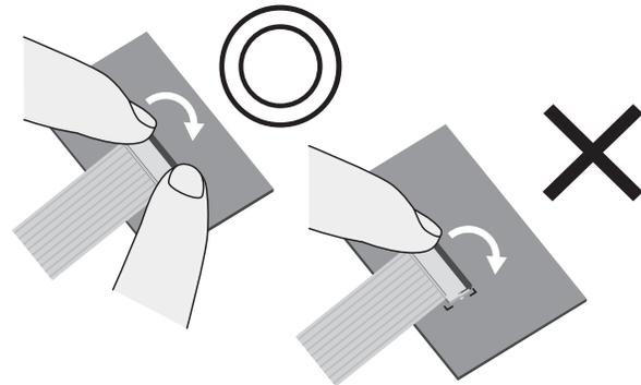
Do not apply force horizontally to the PCB when locking the slider (lever). Doing so may result in damage to the connector or contact failure.
