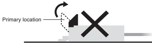
Performing the following action may cause the terminals to change shape or otherwise cause contact failures.
