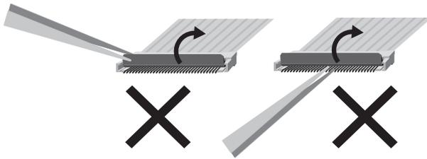
5. When inserting and removing the FPC, be sure to check that the slider (lever) has been unlocked first.
