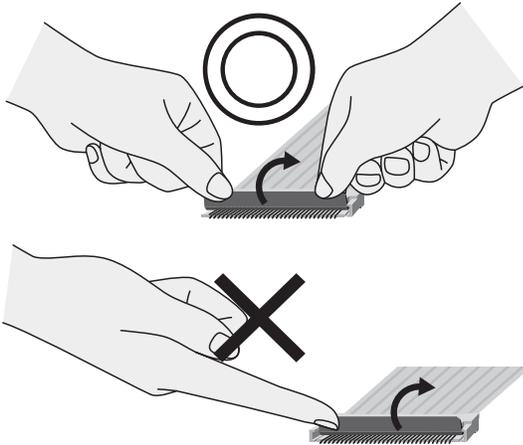
Do not engage the slider (lever) past its initial location during the unlocking process. Doing so may result in damage to the connector or contact failure.
