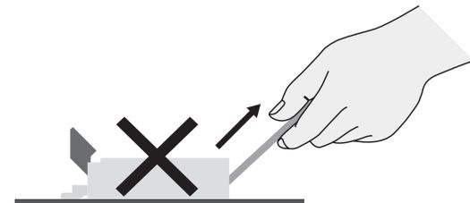
6. Make sure that the FPC has been inserted correctly and not backward.
