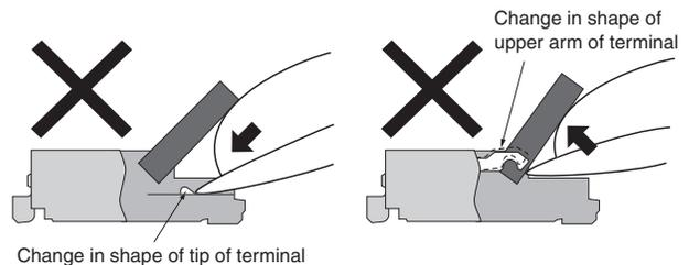
5. Using the FPC in the follow ways may damage the FPC, change the shape of the contacts, or result in contact failure.
