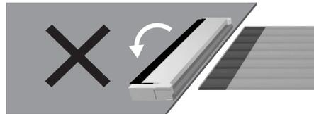
2. Do not lock or unlock the slider (lever) with excessive force. Doing so may result in damage to the connector or contact failure. Do not use a slider (lever) if it becomes detached.
