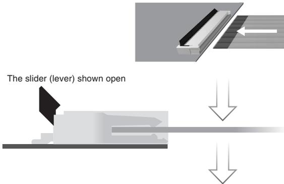
2. Activate the slider (lever) and lock the FPC in place.
