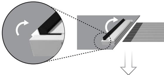
2. Once the lock has been disengaged, pull the FPC out.
