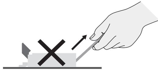
6. Make sure that the FPC has been inserted correctly and not backward.
