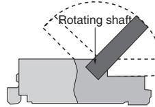
2. The slider cannot be opened to an angle of more than 125°. Do not apply force on the slider beyond that point. Doing so may result in damage to the connector or contact failure. Do not use the slider if it becomes detached.
