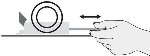
Using the FPC in the follow ways may damage the FPC, change the shape of the contacts, or result in contact failure.
