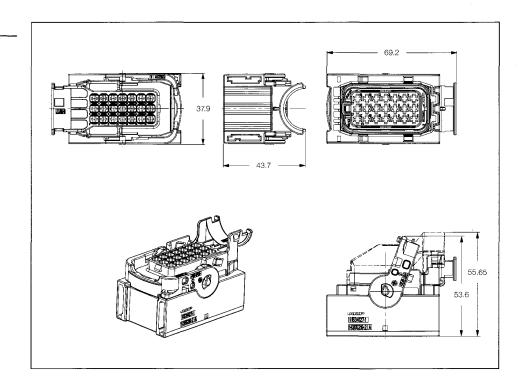
Sealed 2.8 Receptacle Housings with Secondary Locking
