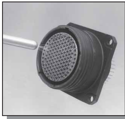
Electrostatic Discharge (ESD) Testing on Tri-Start Filter Connector
