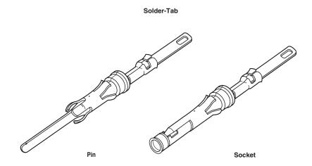
Contact Size 16—Pin Diameter .062 [1.57] (Test Current, 13 Ampere)‡
