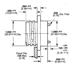
Catalog 82021 Revised 7-07 Dimensions are in inches and millimeters unless otherwise specified. Values in brackets are metric equivalents. Dimensions are shown for reference purposes only. Specifications subject to change.
