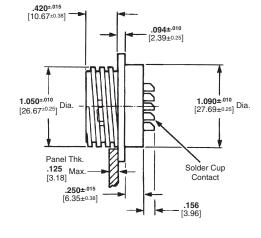
Notes: 1. Connector can be used for pressure bulkhead feed-thru (sealed) applications.
