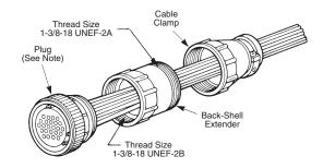
Note: Back-shell extenders can be threaded directly onto plugs or receptacles and will accept cable clamps of the appropriate size (pages 38 and 39).
