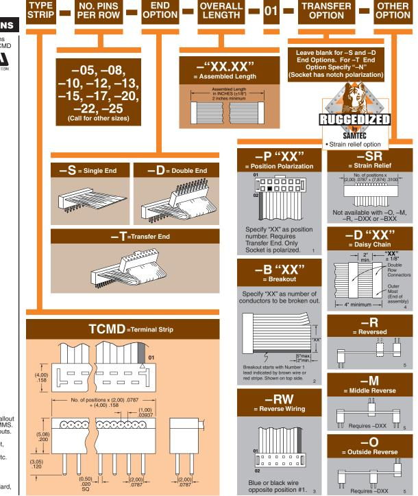
\*Note: Standard TCMD callout will not mate with SMM, MMS. Must use gold plated callouts. (See drawing on web.) When mated with a socket, Wire 1 mates with Pin 2; Wire 2 mates wth Pin 1, etc.
