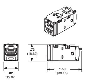
Dimensions are in inches. (Dimension in parenthesis are metric).
