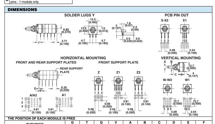
**BUSHINGS** DIMENSIONS mm (± 0.5) **DIMENSIONS INCHES (± 0.02)** 0.150 Ε Leads Z00 3.15 1.85 1.85 3.85 0.071 0.071 0.071 0.071 0.071 Leads Z1. Z2. A. 2.8 3.6 Ε 1.6 1.6 0.063 0.063 0.063 0.063 0.063 0.140 Leads Z0.: 5.08 mm (0.200") Leads A.. Z1. Z2.: 3.81 mm (0.150" Leads X.. Y.. 0.200 0.200 J 6.7 5 5 0.200 0.200 0.200 0.278 0.006 Leads Z0. with Rotary Switch 0.0846 Ε 1.45 0.15 0.15 2.15 0.006 0.006 0.006 0.006
