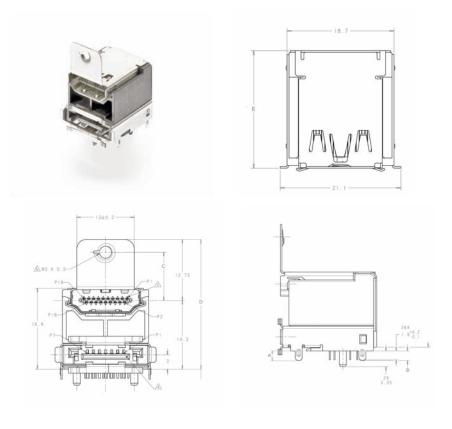
Stacked Right Angle Through Hole Incorporating HDMI Technology over eSATA Technology
