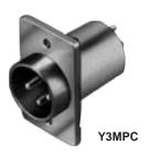
**Series Y(\*)MPC.** Male receptacle for panel or chassis mounting escutcheon. PC terminals and standoffs. Rear of panel mount in .750 inch diameter hole. Maximum panel thickness: 25 inches (6.35 mm); .156 inches (3.96 mm) if YEM escutcheon is used.
