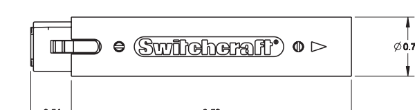
S3F5M 3 PIN FEMALE TO 5 PIN MALE DMX ADAPTER
