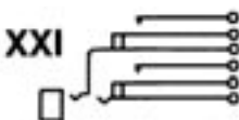
Double open circuit. Isolated switching—separate "make" circuits on both tip and ring. (J2-2A).
