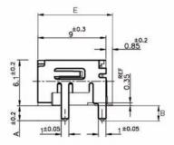
Right Angle Surface Mount Header with Flange (Short Body)
