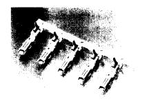
Receptace contacts are manufactured from 0.3 mm [.012 in.] thick material. Uncrimped contact length is 16.5 mm [.650 in.]
