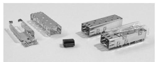
Tyco Electronics offers various termination options for SFP cages, including press-fit, wave solder and IR reflow compatible with tape and reel packaging. The connector is a reliable 20 position interface offered in 0.38  $\mu$ m (15  $\mu$ inch) and 0.76  $\mu$ m (30  $\mu$ inch) gold plating thicknesses. The connector is packaged in tape and reel for pick and place SMT application. The cage material is a copper alloy with nickel subplate and a matte tin finish.
