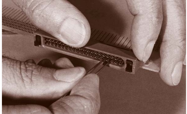
REMOVE DAMAGED CONTACT
