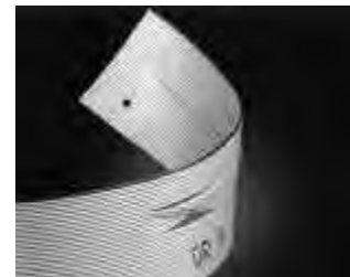
Pre-manufactured Slit-and-Twist Cable (R-CAM 4 only)
