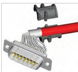
Attach the strain relief around the cable
