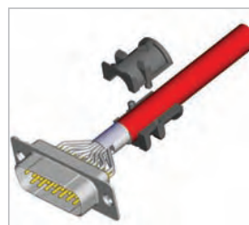
Attach the strain relief around the cable
