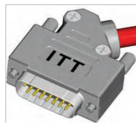
Assemble the other half (screwing force: 100-120 Ncm)
