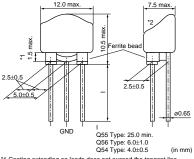
\*1 Coating extending on leads does not exceed the tangent line. Exposed electrode, if any, is covered by solder, etc. \*2 There should not be the exposure of the ferrite bead if a hole is in top of filter, the ferrite bead should not be exposed.
