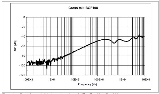
Figure 4 Typical cross talk between two channels ( $Z_S = Z_L = 50 \Omega$ ,  $V_R = 0 V$ )
