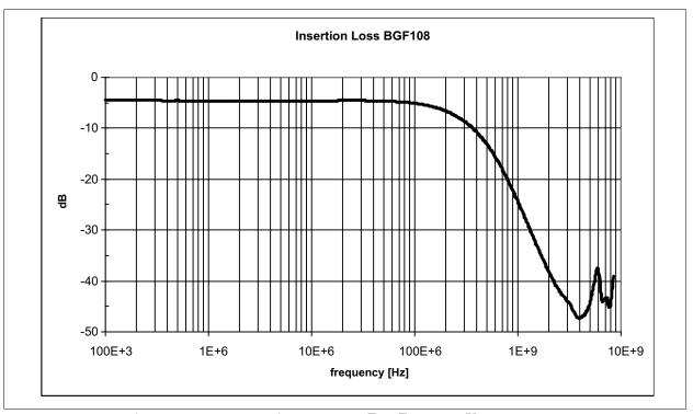
Figure 3 Typical filter characteristics of on channel ( $Z_S = Z_L = 50 \Omega$ ,  $V_R = 0 V$ )
