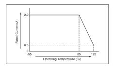
NFM31P series is EMI suppression filter for power lines of high speed IC with high capacitance (27uF) and large rated current (6A) in 3.2x1.6mm chip size, which is realized using Murata's high level multilayer processing technology.
