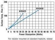
For resistor mounted on standard heatsink, related to power dissipation
