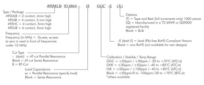
Part Number Examples: Freq 5.1234MHz, ±30ppm calib, ±30ppm stability, -20 to +70°C, 16pF = 49SMLB05.1234-16GGC
