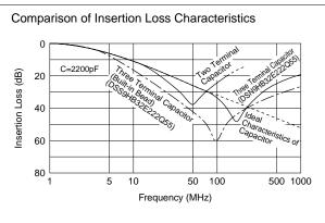
A three terminal capacitor has a higher self resonance frequency than a general two terminal type and exhibits effective noise suppression at high frequency.
