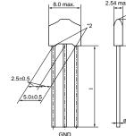
\*1 There may be a hole on the top of ferrite beads, which causes no characteristics deterioration. \*2 Bottom of the ferrite beads may not be level with each other.
